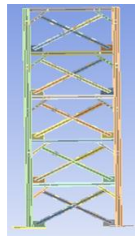
Fig -5: Modal of double knee braced frame
