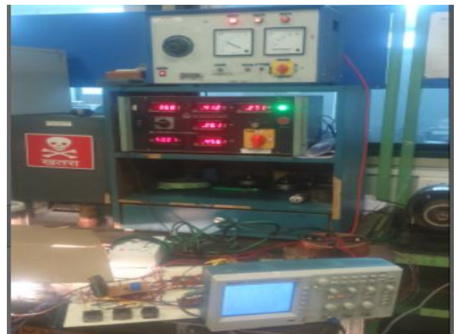
Fig. 6 Hardware implementation of Three phase to Two Phase Matrix Converter.
