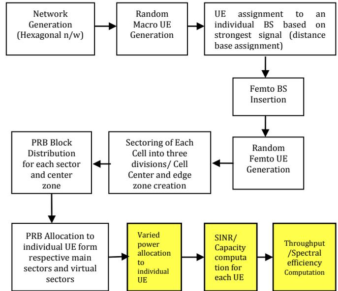
Fig- 3: Proposed method of varied power distribution
