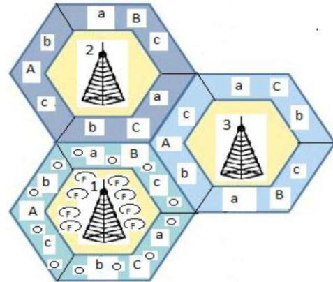
Fig -1: Femtocells deployment in Macrocells
