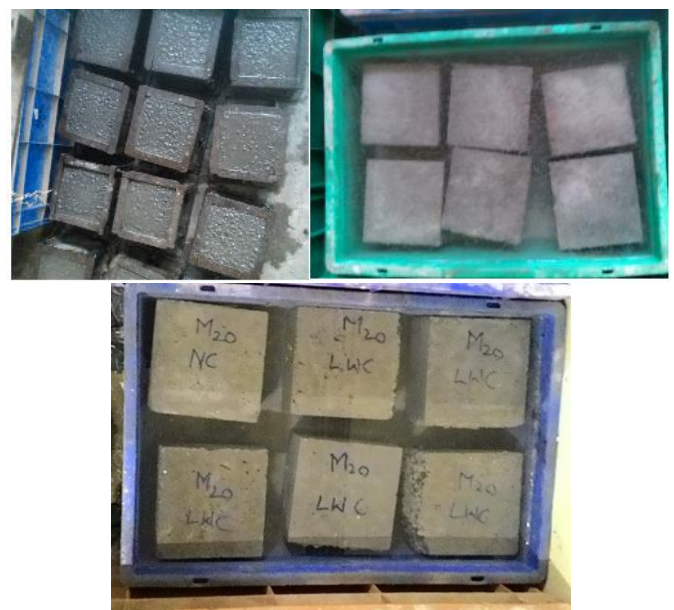
Fig- 4: Casting and curing of Cube specimens
