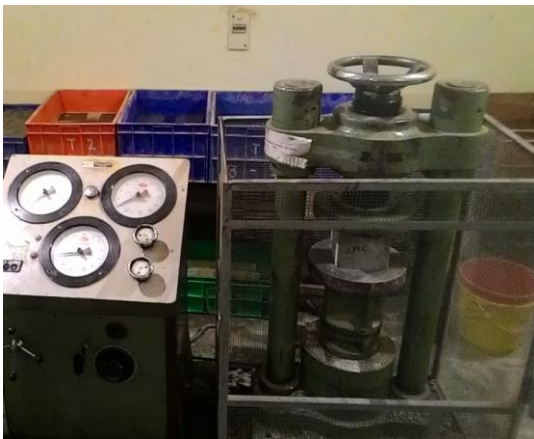
Fig -5: Testing of cubes in Compression testing machine
