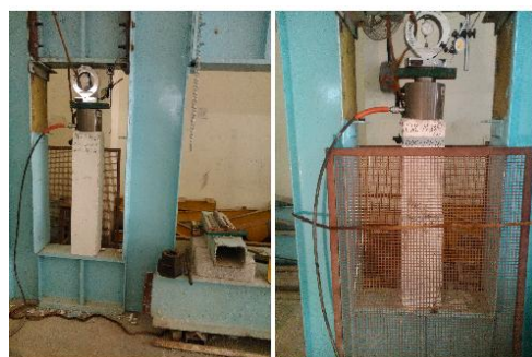
Fig -9: Loading arrangement for columns
