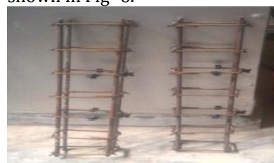
Fig -6: Reinforcement details of Column
