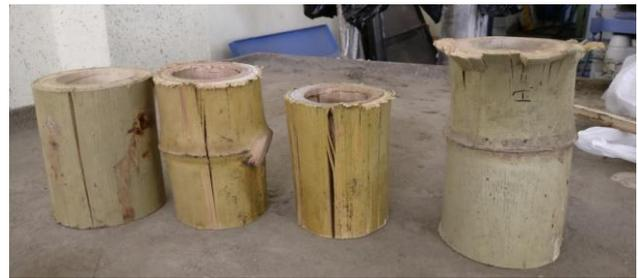
Figure 8: failure of bamboo by compression test
