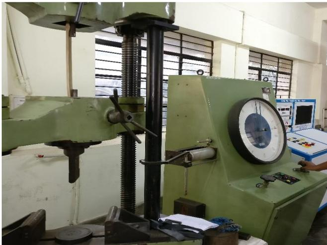
figure 5: tensile test on bamboo
