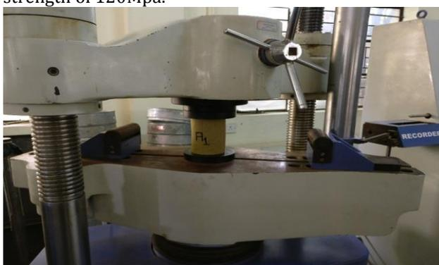
Figure 7: compression test on bamboo
