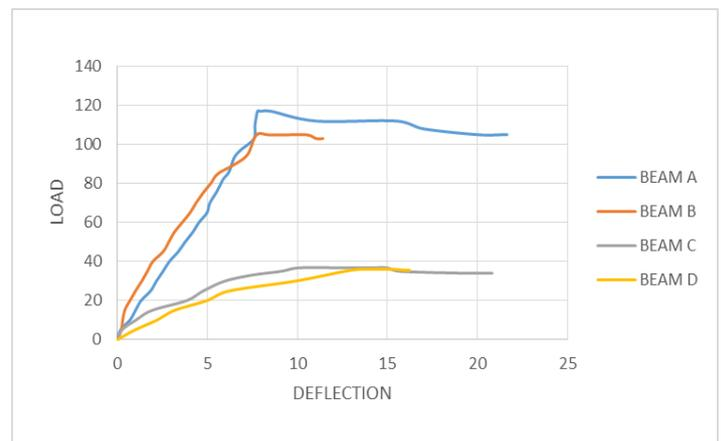
From the above graph, it is clearly showing the pattern of cracking and the failure of differently reinforced beams.it also explains the behaviour of beams under the stresses. BEAM B found to be more successful and can be used as singly reinforced beam
