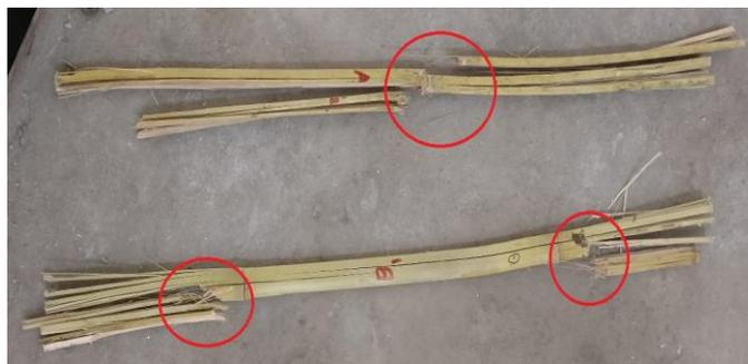
Figure 6: Failure of Bamboo by Tensile Test
