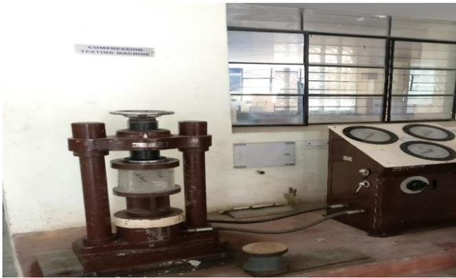
Figure 10: Test Setup to check Compressive Strength
