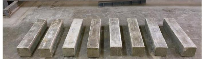
Figure 12: Beams Ready for testing
