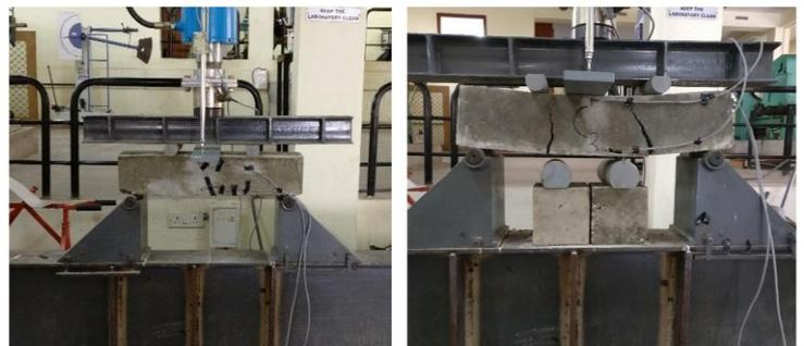
Figure 13: Loading frame setup Figure 14: Flexure failure of beam
