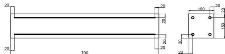
Figure 4: schematic representation of bamboo reinforcement BEAM A
