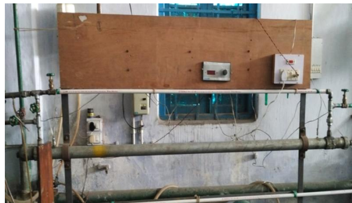
Figure 2: Experimental setup of triangular baffled heat exchanger
