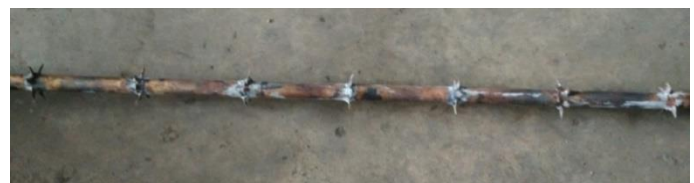
Figure 4: Triangular baffles with 100 mm pitch on cu-pipe
