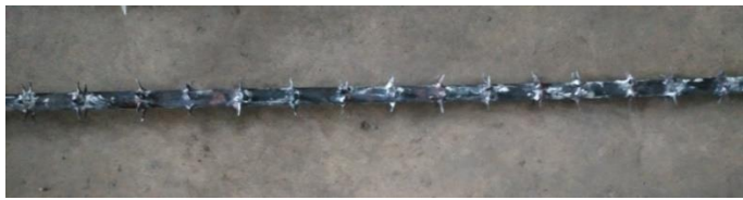
Figure 5: Triangular baffles with 50 mm pitch on cu-pipe
