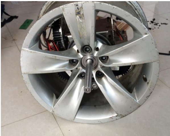
Fig -6: Implementation of designed transmission system in side wheel of motorcycle
