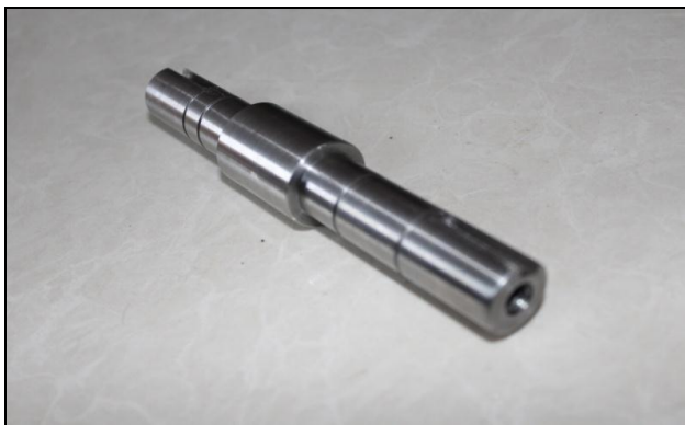
Fig -4: Intermediate shaft (Jackshaft)
