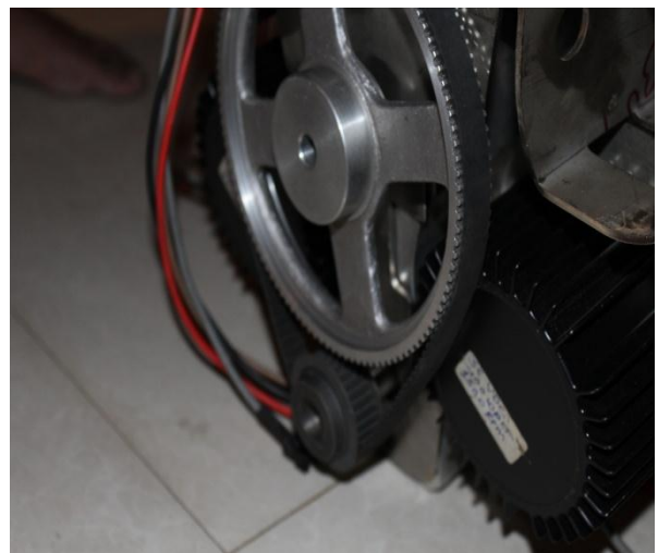
Fig -5: Primary stage and Secondary stage transmission system
