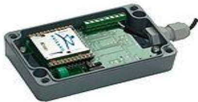
Fig. 1.1 Data logger storing technical and sensor data
