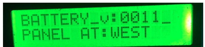
Fig5: Monitoring the solar Panel moving in west direction and Battery voltage
