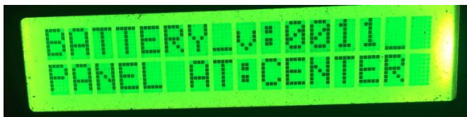
Fig8: Monitoring the solar Panel moving in Center direction and Battery voltage
