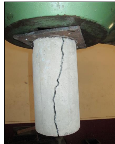
Fig -5: Failure pattern for 300 mm embedded length (splitting)
