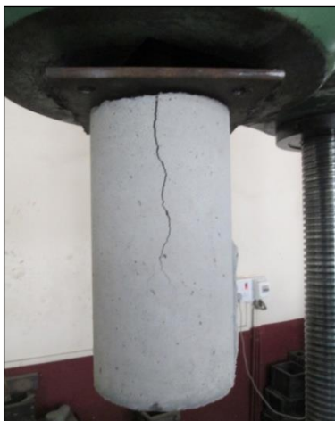
Fig -4: Failure pattern for 150 mm embedded length (splitting)
