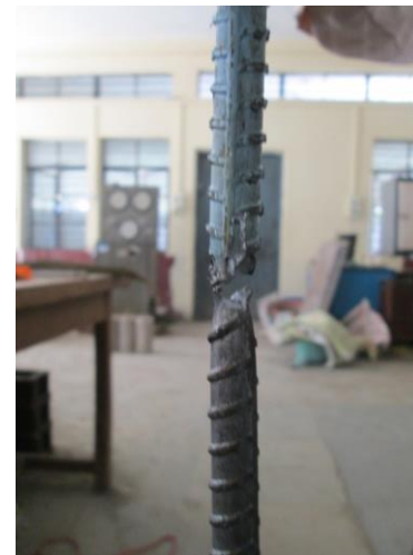
Fig -6: Failure pattern for 300 mm embedded length (steel rupture)
