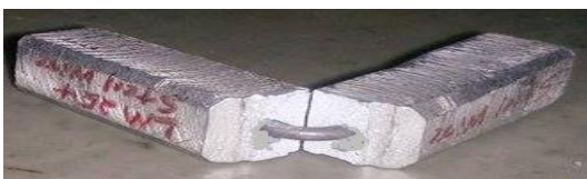
Figure 4.8 –LM 25 Al alloy reinforced with steel wire after charpy test
