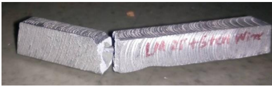
Figure 4.6 –LM 25 Al alloy reinforced with steel wire after Izod test
