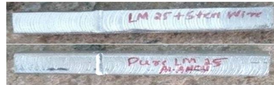
Figure3- Izod test specimen Dimensions in mm (ASTM E23) Finish requirements 2 μm on notched surface and opposite face; 4 μm on other two surface.
