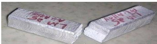
Figure 4.7 –LM 25 Al after charpy test 2) LM 25 Al Alloy reinforced with steel wire.
