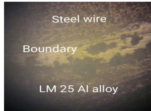
Fig4. 2-Microstructure [Magnification: (450X) x4]
