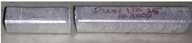
Figure 4.5 –LM 25 Al alloy after Izod test 2) LM 25 Al alloy reinforced with Steel
