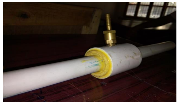
Fig -2: Vortex tube with nozzle setup
