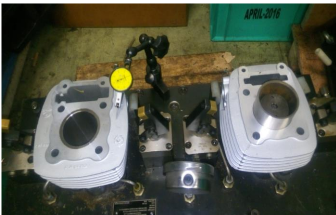
Fig-15: Dial gauge indicator mounted on fixture
