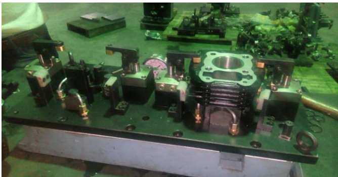
Fig-14: Manufactured fixture with cylinder block clamped
