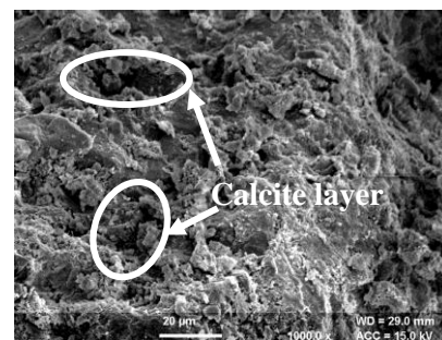
Figure -7 (c): Bacterial Concrete (Urea Medium)
