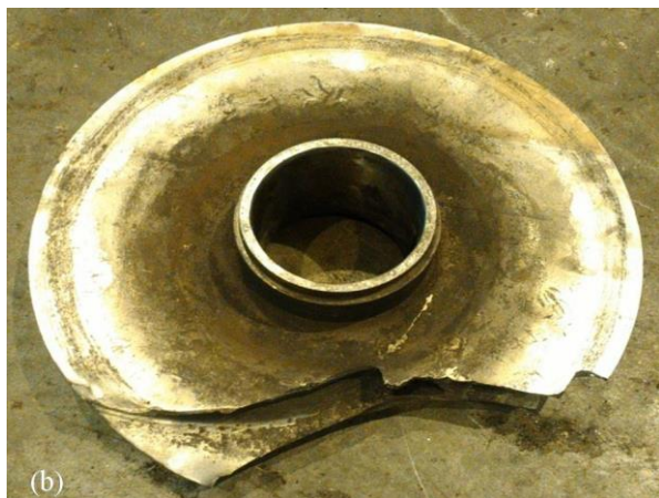
Fig-1 (b) Damaged impeller
