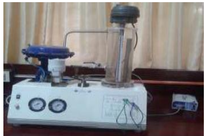
Fig 1: The Liquid Level System VLPA-101-CE
