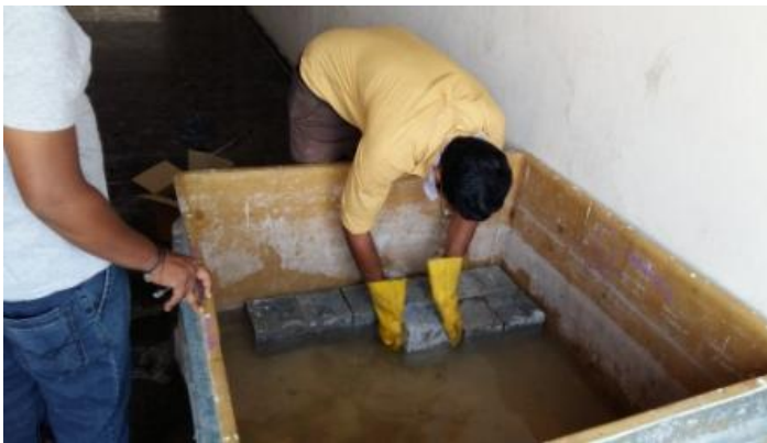
Fig 3: Immersion of specimens in acid tank
