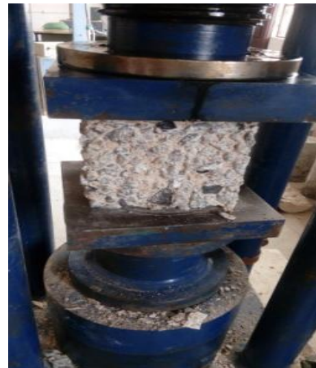
Fig 2: Testing of cubes for Compressive strength
