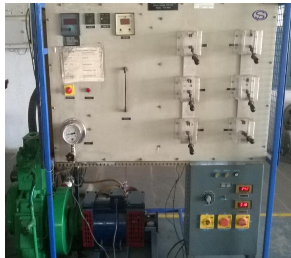
FIG 2: 4 Stroke single cylinder diesel engine set up with generator loading
