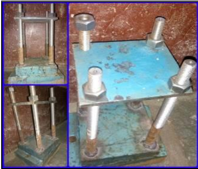
Fig. 4. Fixed Support assembly
