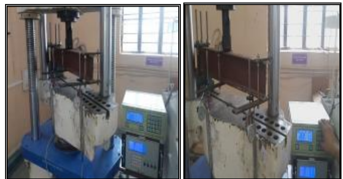
Fig.12. Lateral torsional buckling on NPI-125 (Plane)
