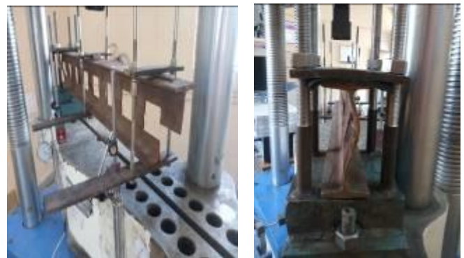
Fig.10. Lateral torsional buckling on NPI-125 (Square)
