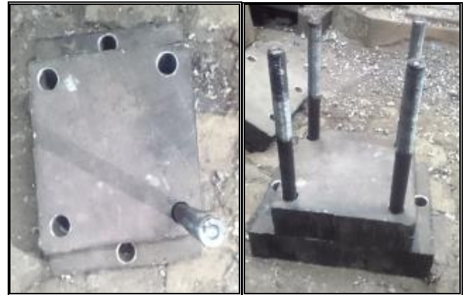
Fig. 5. Fabrication of Fixed Support assembly
