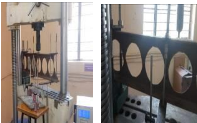
Fig.8. Lateral torsional buckling on NPI-125 (Circular)
