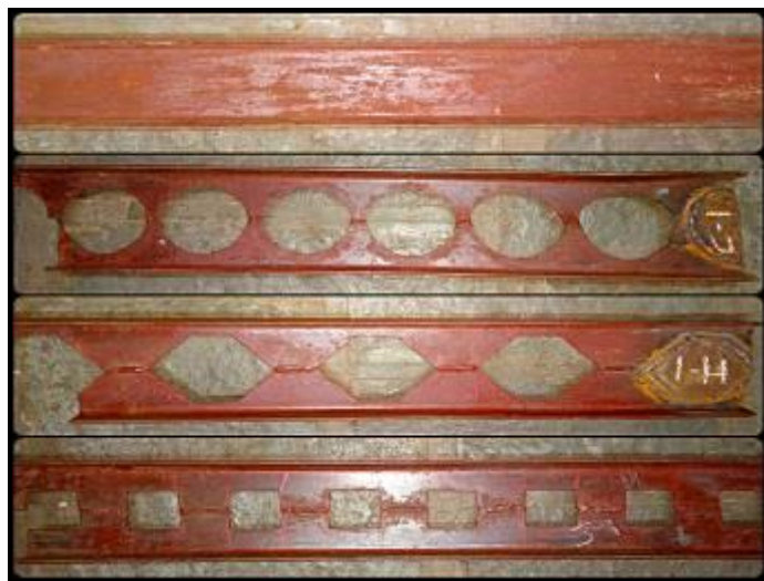
Fig. 3. Shape of Castellated beam
