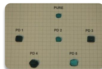
Fig1. Photograph of the grown Pure and Doped NSH crystals.
