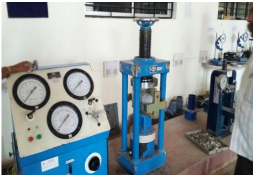
Fig 4.3 Split tensile test
