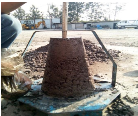
Fig 4.1 Slump cone test
