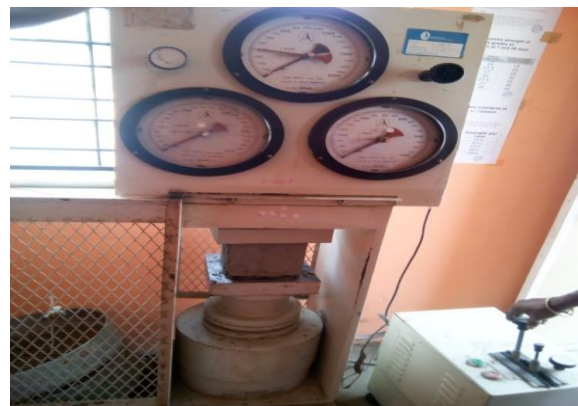
Fig 4.2 Compressive strength test
