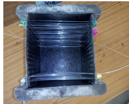
Figure: 3 Placing of optical fibre
