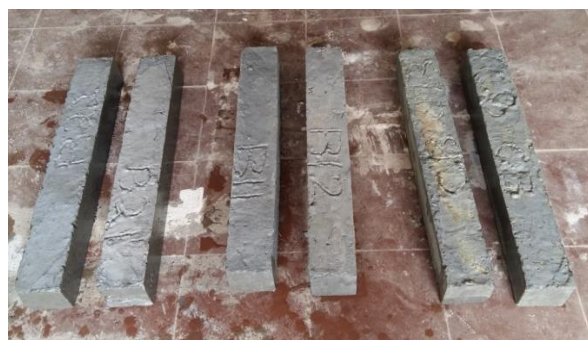
Fig -2 : Cast beam specimens
