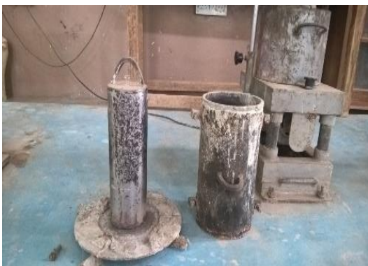
Fig -3: MS moulds for casting hollow cylinder
