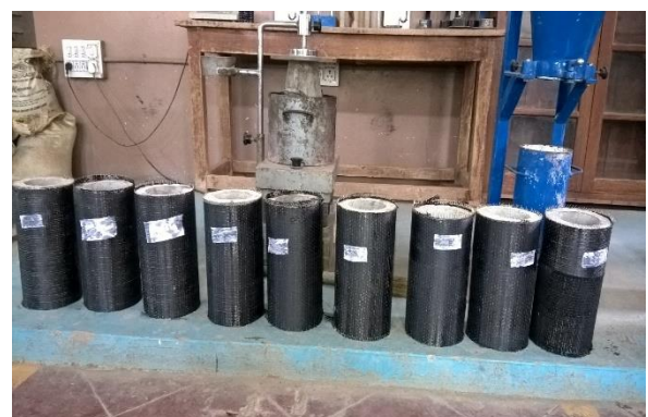
Fig -5: Confined hollow cylinder
