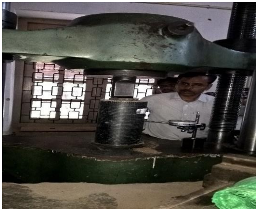
Fig -6: CFRP confined hollow concrete testing in UTM
