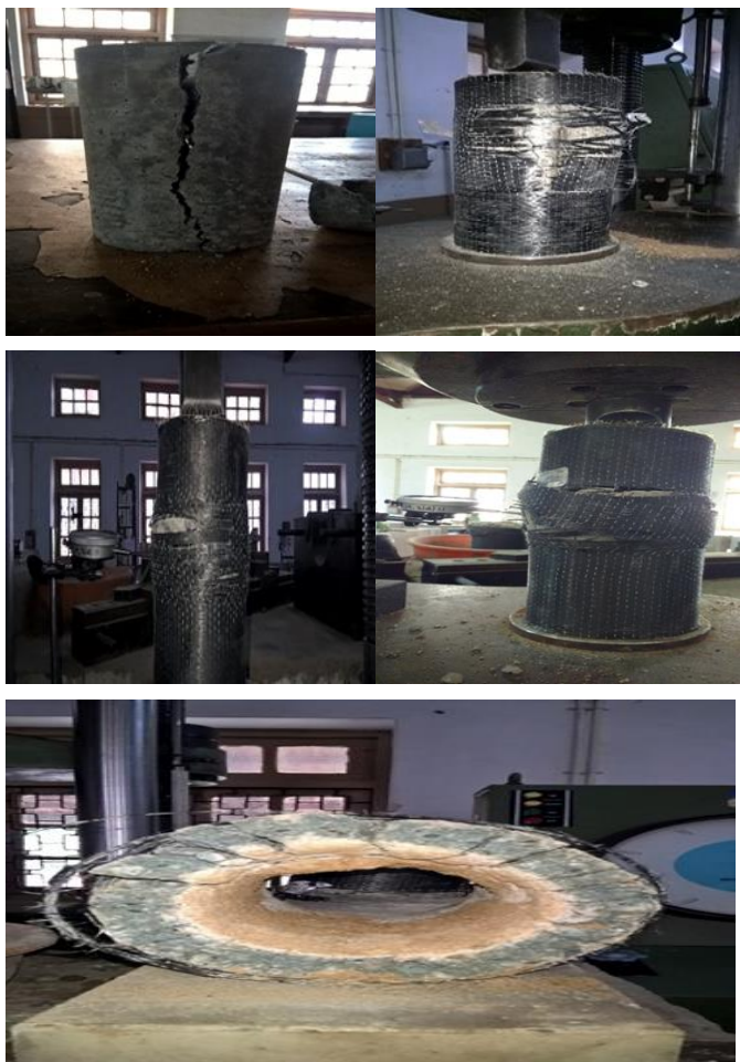
Fig -8: Failure pattern of unconfined and 1/2/3 layer CFRP confined hollow concrete cylinders
