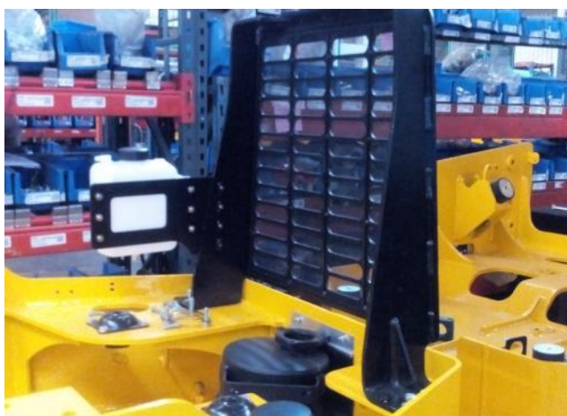
Fig- 10 Assembly of Bracket on assembly line.
