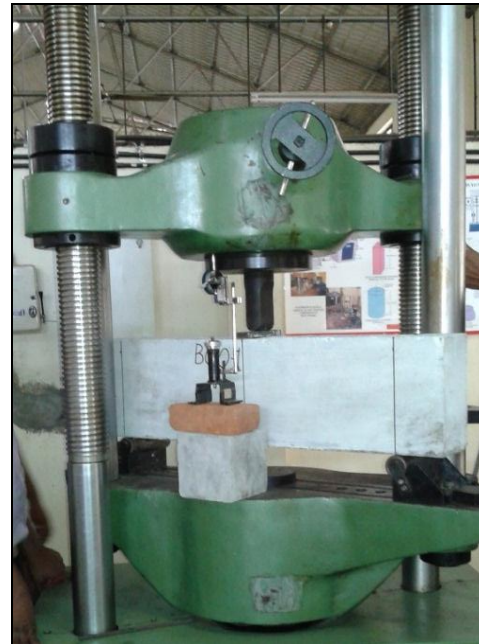
Fig - 5 : Test setup for beams
