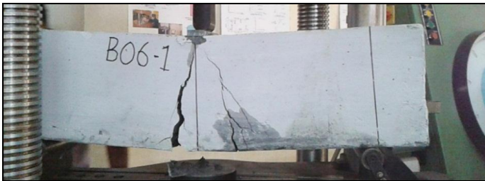
Fig - 8: Cracking pattern of B06
