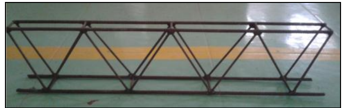
(b) Reinforcement cage for specimen B06
