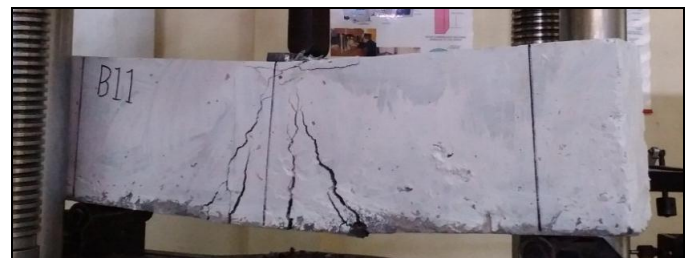
Fig - 7: Cracking pattern of B11
