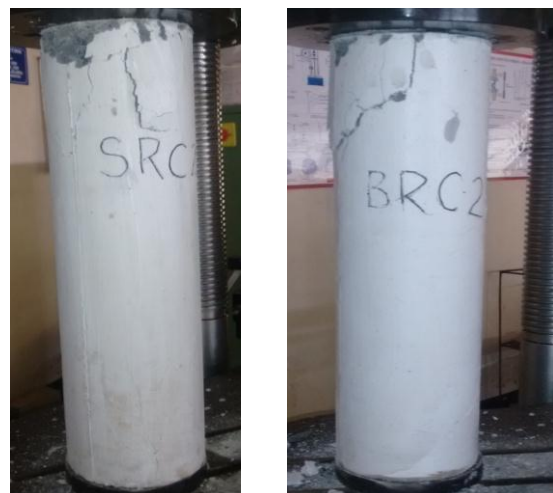
Fig -9: Failure pattern of column SRC1 and BRC 2
