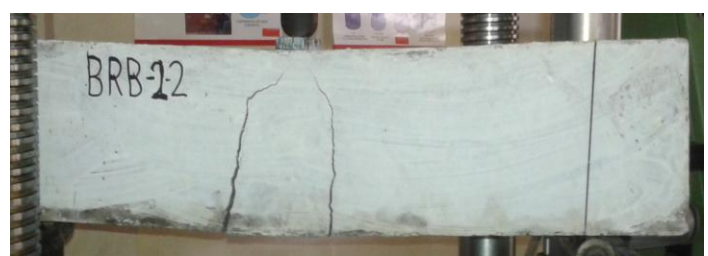
Fig -6: Crack pattern of beam BRB2-2
