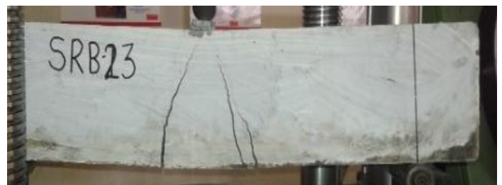
Fig -5: Crack pattern of beam SRB2-3
