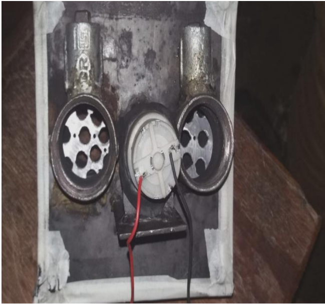
Fig. 2 side view of Heat Wheel Set up with inlet outlet pipe openings
