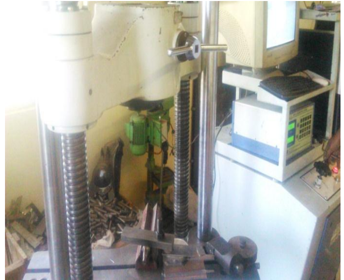
Fig.4- : Shear Test Set-Up on Universal Testing Machine
