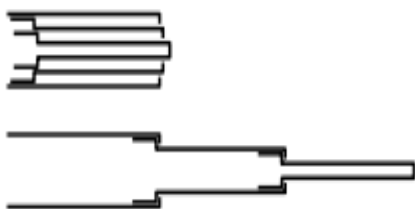
Fig -2 showing the telescopic principle, an object collapsed (top) and extended (bottom), providing more reach.
