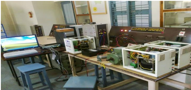
Fig 2: Experimental set up of 10-HP three phase Induction motor Stator inter turn fault detection.
