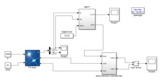
Fig-4: Simulation of PV panel with MPPT
