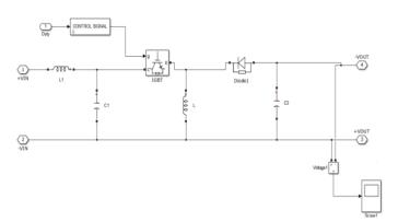
Fig-3: Buck boost converter
