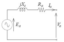
Fig -10: Equivalent circuit diagram of PMSM
