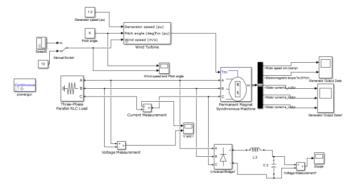
Fig -11: Simulation of wind turbine with PMSG
