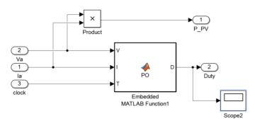
Fig-6: Simulation of P&O algorithm
