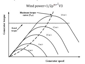
Fig -9: Characteristics of Wind Turbine
