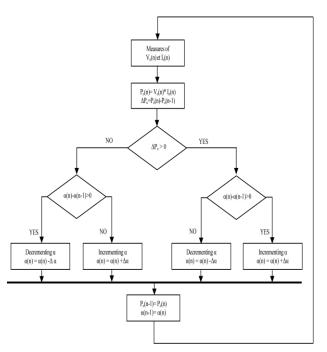
**Fig-2:** Flowchart of P&O algorithm with the output sensing method.
