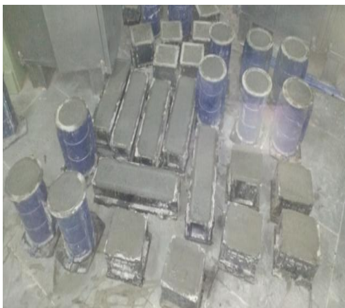
Fig -2 Moulds After Filling of Concrete
