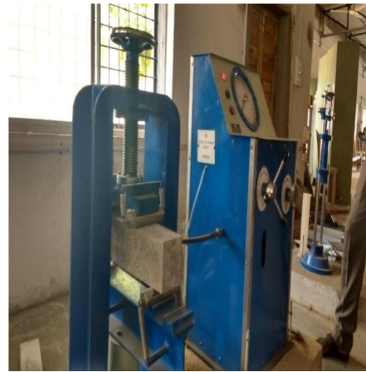
Fig -3 Testing of prism in flexural Testing Machine
