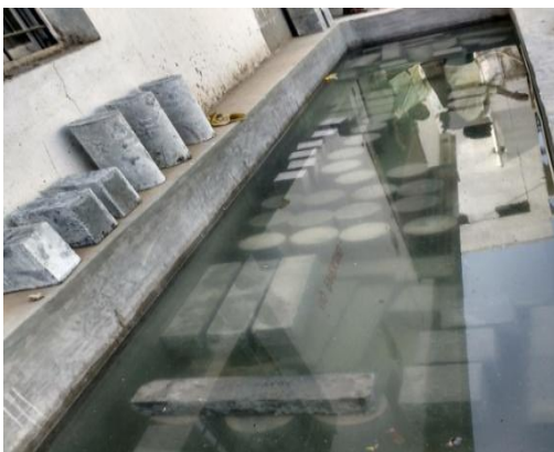
Fig -2 Specimens are Kept For Curing in Curing Pond
