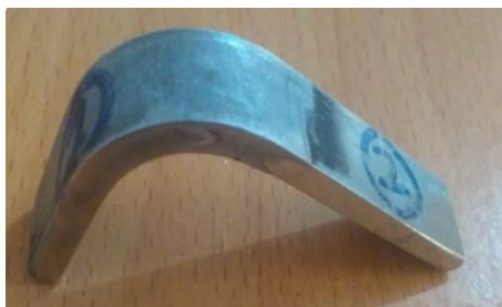
Fig -14: Bend test
