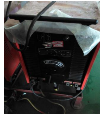
Fig -2: Ador welding transformer
