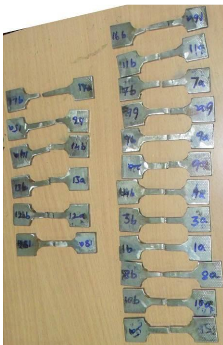
Fig -4: Specimens after testing
