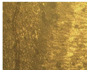
Fig -11: HAZ of base metal SDSS 2507
