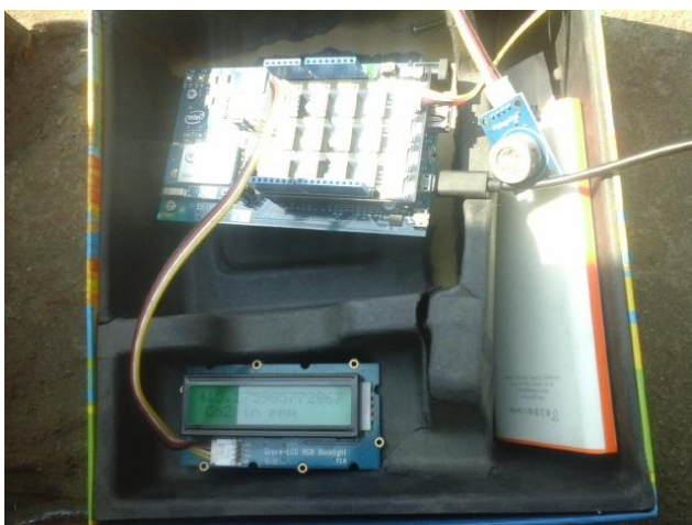
Fig-2: Intel Edison Board connected with Mq7 gas sensor
