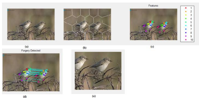
Fig -3: (a) Host Image (b) Segmented Image (c) Feature Extraction using SIFT (d) Feature Matching (e) Forgery Region Extraction
