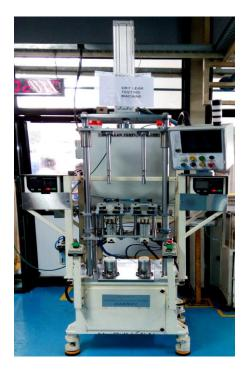
Fig-2: Dry Leak Testing Machine
