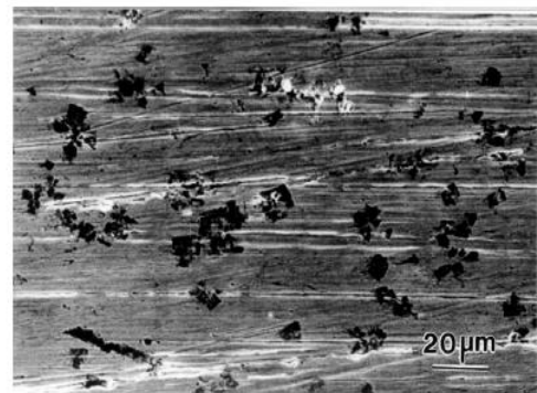
Figure 2. SEM micrograph of Fe-TiC composites showing micro network of TiC particles
