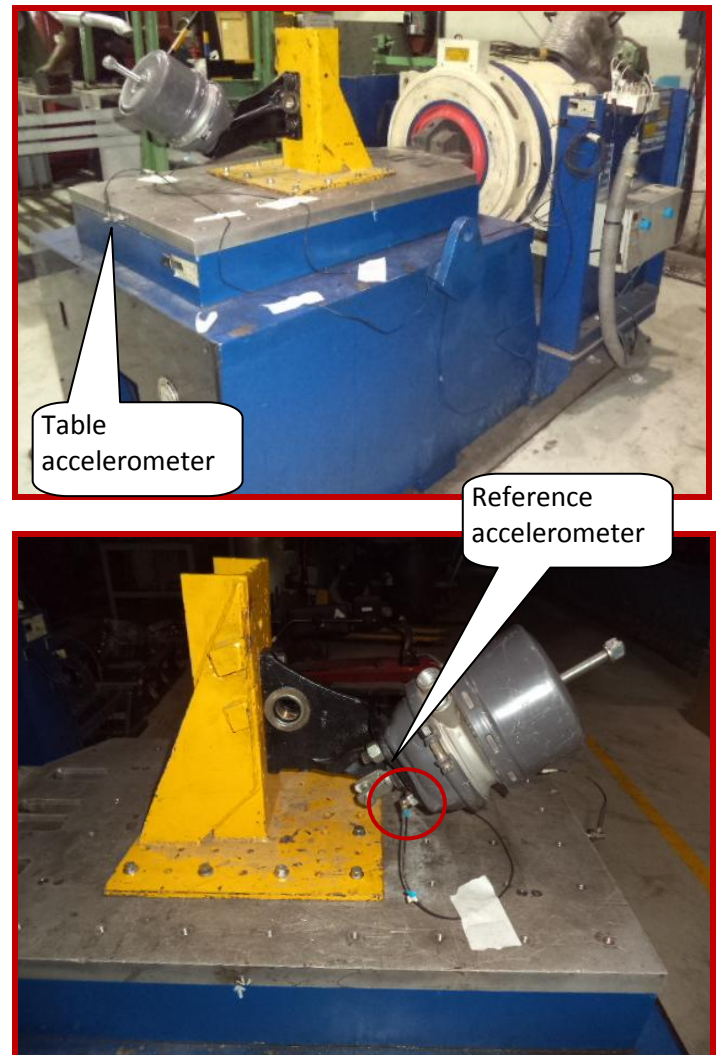
Figure 6 -Natural frequency detection test setup
