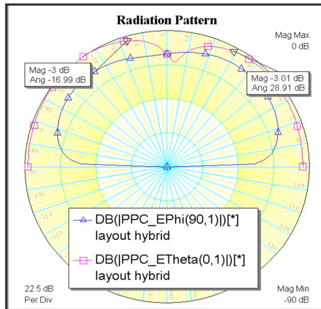
**Figure 7: Half power beamwidth**
