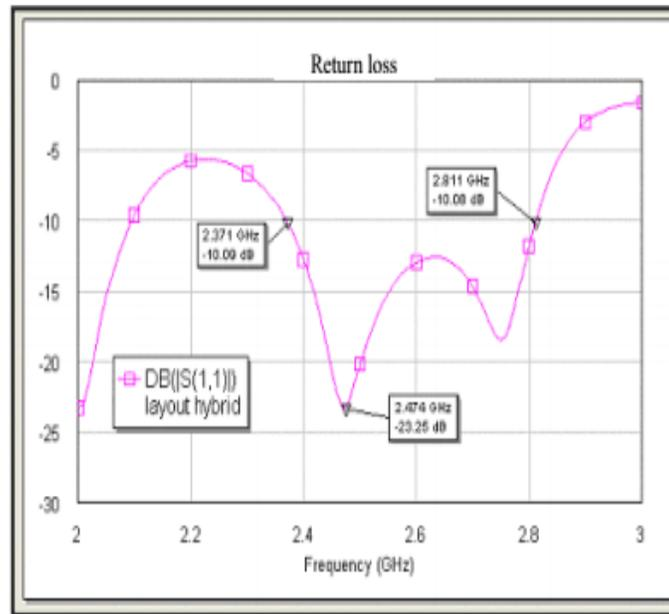
**Figure 4: Return loss of the microstrip patch antenna**
