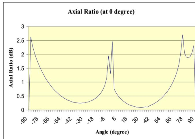
**Figure 10: Axial ratio for the microstrip antenna**
