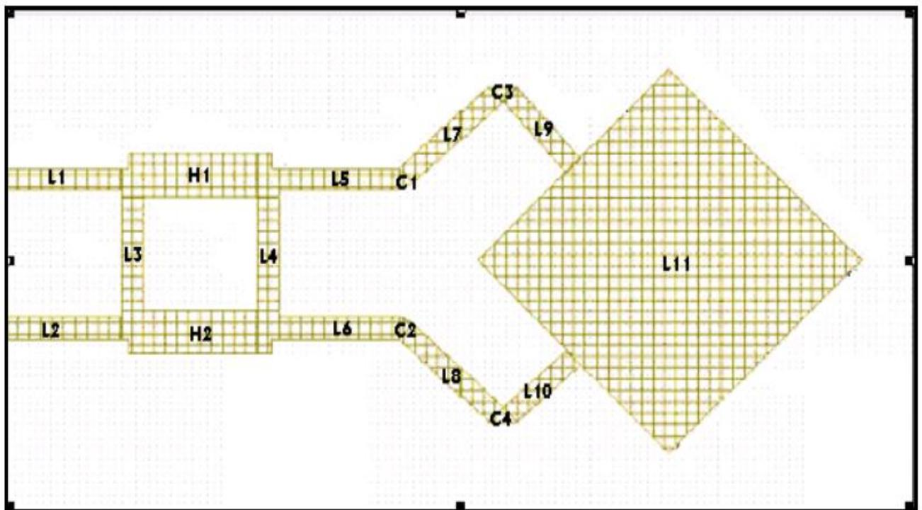
Figure 2: Layout of the Microstrip Patch Antenna
