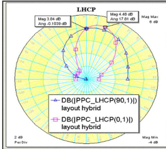
**Figure 8: Left hand circular polarization**
