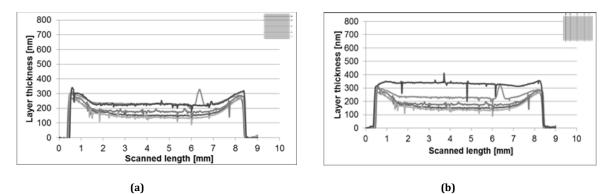
**Figure 2:** The surface profile of the bottom silver electrode without corona pretreatment at a drop space of 25  $\mu$ m in (a) print direction (b) across print direction; with representation of five scans from dark grey color to light grey color for first to last scan respectively.
