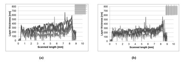
**Figure 3:** The surface profile of the bottom silver electrode with corona pretreatment at a drop space of 25  $\mu$ m in (a) print direction (b) across print direction; with representation of five scans from dark grey color to light grey color for first to last scan respectively.
