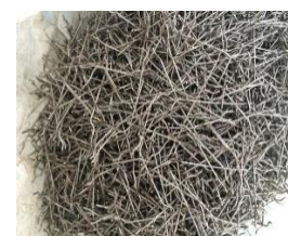
Fig.6- AR Glass fibres. fig.7- Steel Fibres
