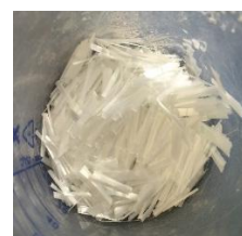
Fig.6- AR Glass fibres. fig.7- Steel Fibres
