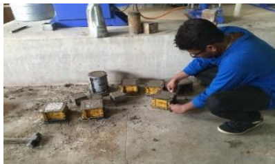
Fig.9- Mold used for casting specimens.
