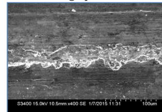
Fig-3: SEM for Speed 4m/s, 4Kg load, H.T. 3 Hr 100X
