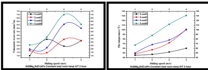
**Fig -5:** Homogenized for 3 hr, (a) Speed v/s Volumetric wear rate, (b) Speed v/s Interface temperature
