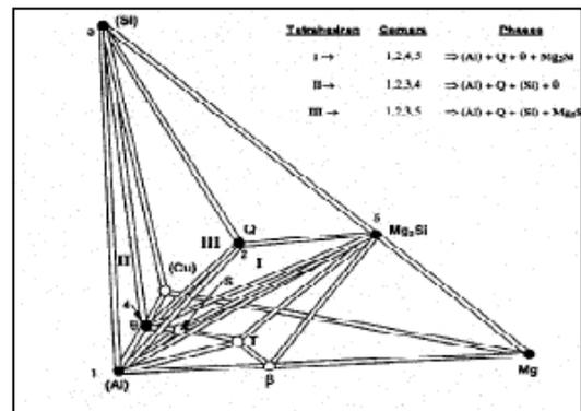
**Fig -1:** Line diagram of stable equilibrium phase fields in Al-Mg-Si-Cu system at normal aging temperatures
