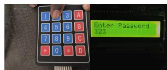
Fig-6 4x4 keypad and LCD display
