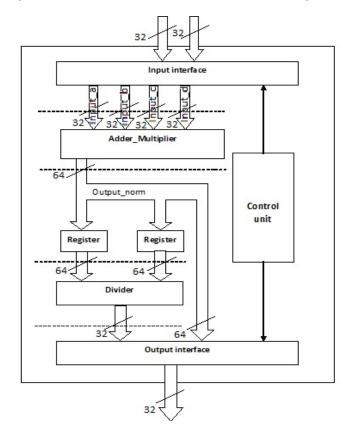
Fig -3: Block diagram of CAALU module
