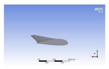
Fig.4 : Wing with Modified Profile & Dihedral Angle
