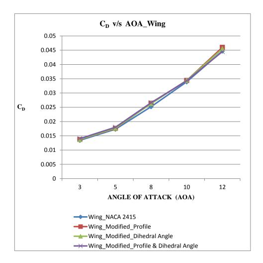
Fig.7 : Drag Coefficient (C<sub>D</sub>) at various angle attack
