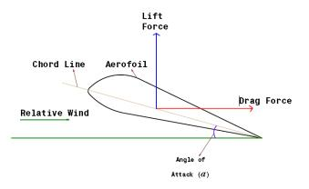
Fig. 2 : Lift and Drag Force
