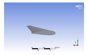
Fig.3 : Wing with NACA 2415
