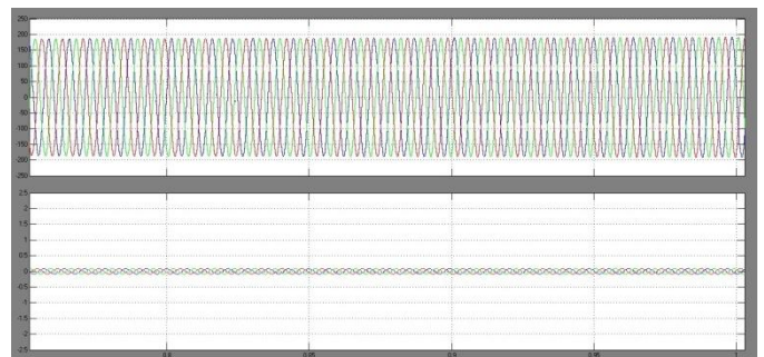
Fig-12: Output voltage and current of PMSG ( x axis= 0.8 s/div, y axis= 50 V/div, 0.5 A/div)
