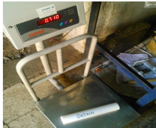
Fig No.6-Weight measurement of DELRIN Roller
