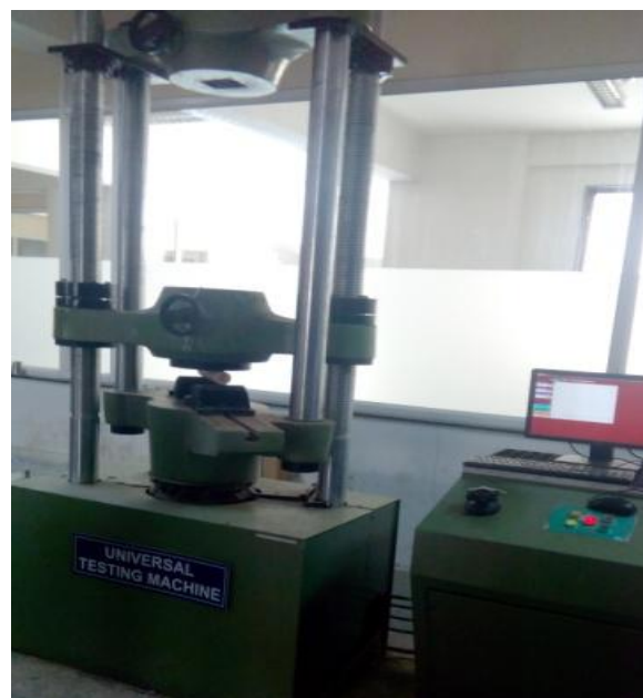
Fig No.-8 Testing of materials using UTM
