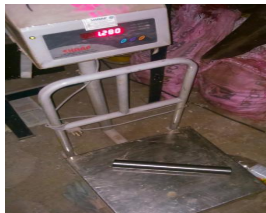
Fig No.7-Weight measurement of Existing (M.S.) Roller
