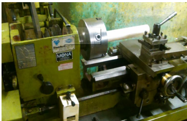
Fig No 5- Manufacturing of Roller using Lathe Machine.
