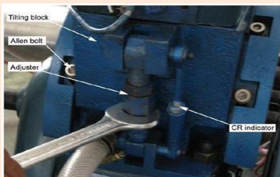
Fig 3.2 Compression Ratio Setting
