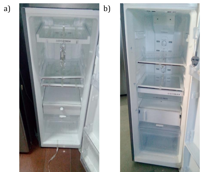
Fig -5: Placement of vacuum compartment in refrigerator for a) Concept 1 b) Concept 2
